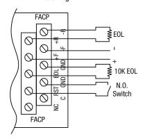
Fig. 12 - Normally Closed trigger input (Non-Latching).
