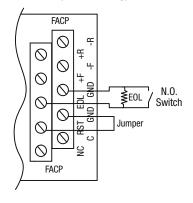
Fig. 15 - Normally Open trigger input (Latching).
