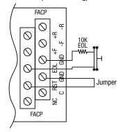
Fig. 13 - Normally Closed trigger input (Latching).
