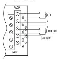
Fig. 11 - Polarity reversal input from FACP signaling circuit output (polarity is referenced in alarm condition).
