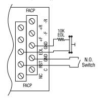
Fig. 14 - Normally Open trigger input (Non-Latching).
